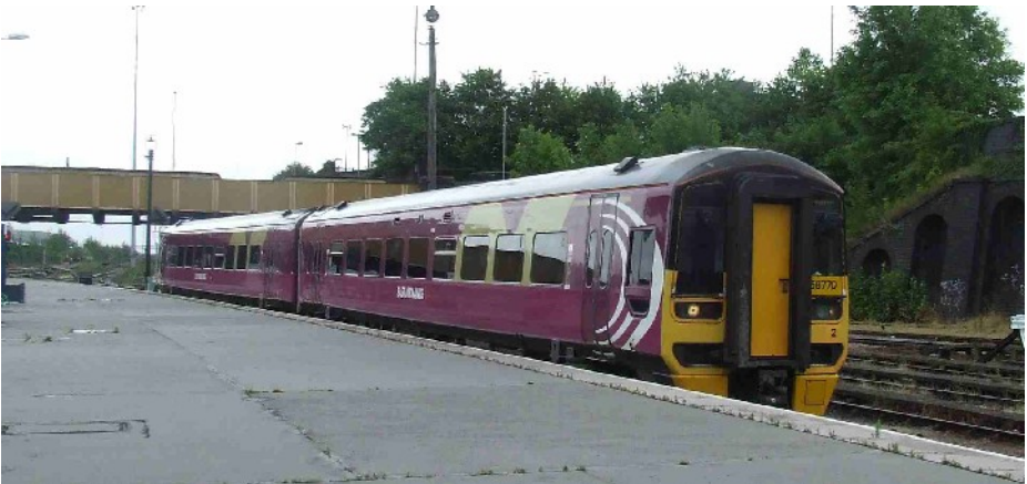
The nomadic lives of the former Heaton based class 158 units displaced from trans-pennine services by class 185's can be seen in the livery carried by 158770 seen at Leicester on 16 July 2009. The bottom half of the original Northern Spirit purple livery with a large gold N was covered in purple vinyl for First Trans Pennine. Subsequent transfer to Central saw the lower panels stripped back to plain purple, revealing a lighter less faded shade than the upper panels, plus the addition of fleet names and the curly big C logos at the carriage ends. A further transfer to East Midlands Trains has seen the fleet name replaced thus leaving the unit showing evidence of four operators liveries. Take a look on the Society's web site to see all the pictures in glorious colour.
