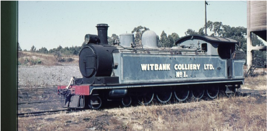
A North British 4-10-2 tank engine built in 1927 to a Natal Government Railway design seen in industrial use.
