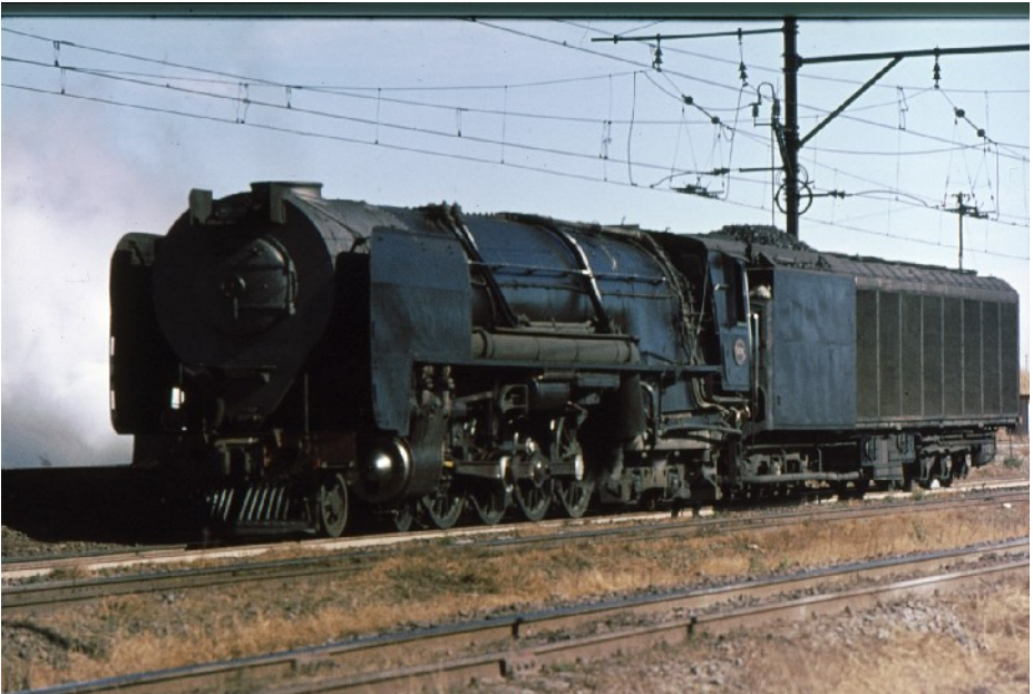
One of the imposing and impressive class 25 4-8-4 condensing locomotives built in 1953/54 by North British (loco's) and Henschel (tenders). Photographed at Kimberley in 1976.
