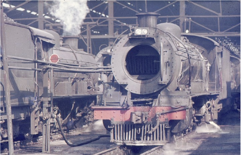
Just like old times in the UK! A typical scene as two class 12A's receive boiler washouts at Germiston depot. Colin Stone
