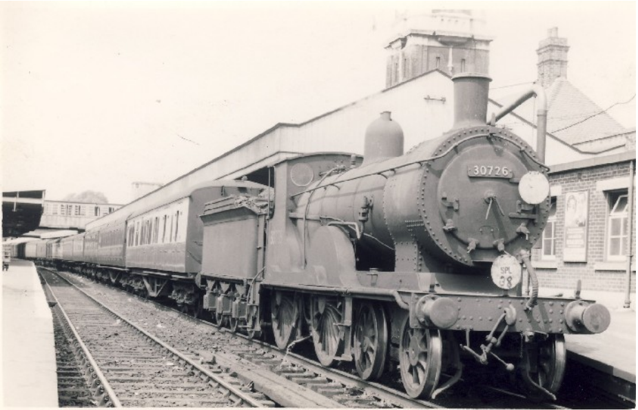
Drummond T9 30726 on ECS at Southampton Central on 24 July 1959. This was one of the locos that received a six wheel tender, and was withdrawn less than a month later in August 1959. WRS C88
