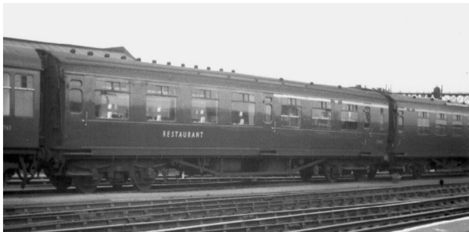
A Restaurant/First from the no. series 7677 – 7687 photographed at Clapham Junction in 1965; note the extended sheeting covering the solebar. It is coupled to the first class end of a composite but the restaurant section has been downgraded to second class. The Kitchen/Restaurant car in the 6 coach set has been replaced by Mk1 RB 1763. Photo copyright RCTS, Mike Stollery collection
