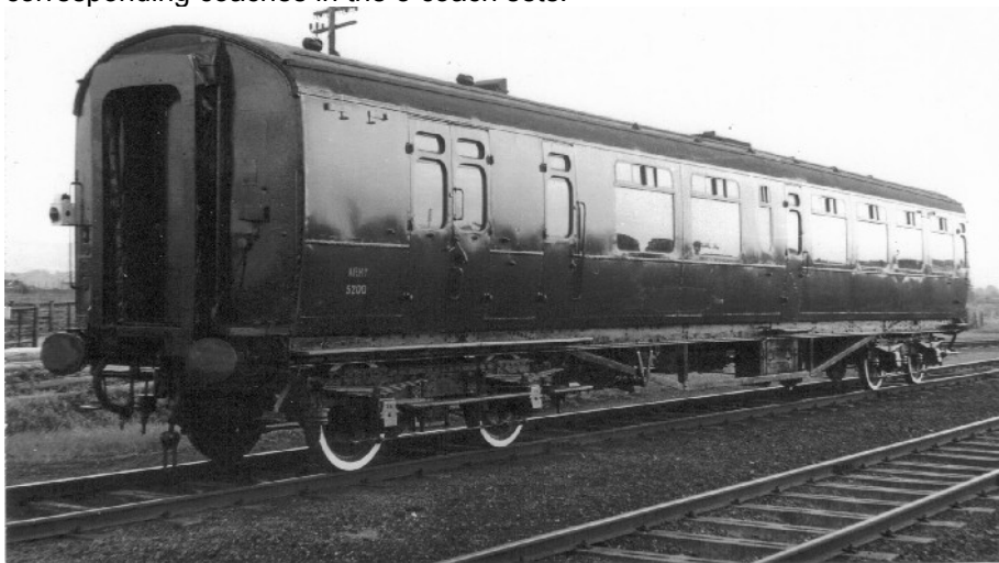
Bulleid Brake Third 4365 in Army service as 5200. When out-shopped in early 1948, it formed one end of Restaurant Set 298 and had the extended sheeting as on the Restaurant/First shown below. As pictured, however, it is identical to the BTKs in the 3 car sets 770 – 793 and 2 car sets 63 – 75. Photo Mike Stollery collection.
