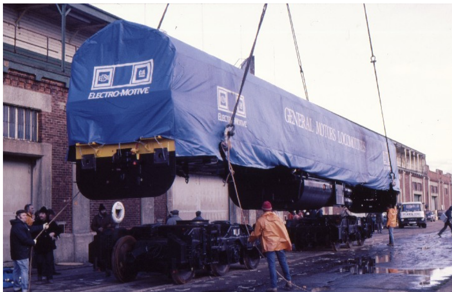
The locomotives were transported off their bogies which were unloaded separately. Here we see 59004 being lowered on to its bogies on the dockside at Southampton.
