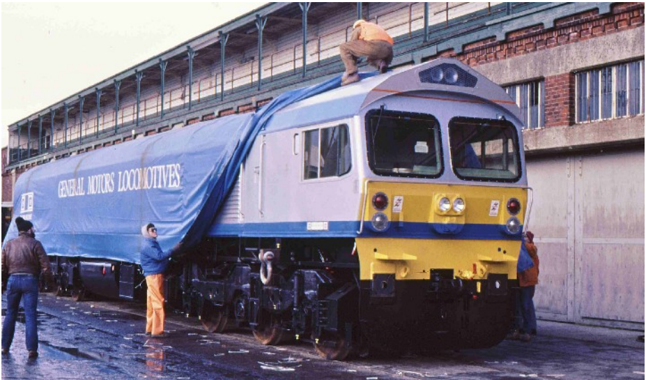
The sheets are carefully rolled back from 59002 on the dock side at Southampton. The crane lifting eyes are still attached to the frames above the bogies, and it is interesting to see that the locomotive is not yet fitted with buffers and has a conventional draw hook.
