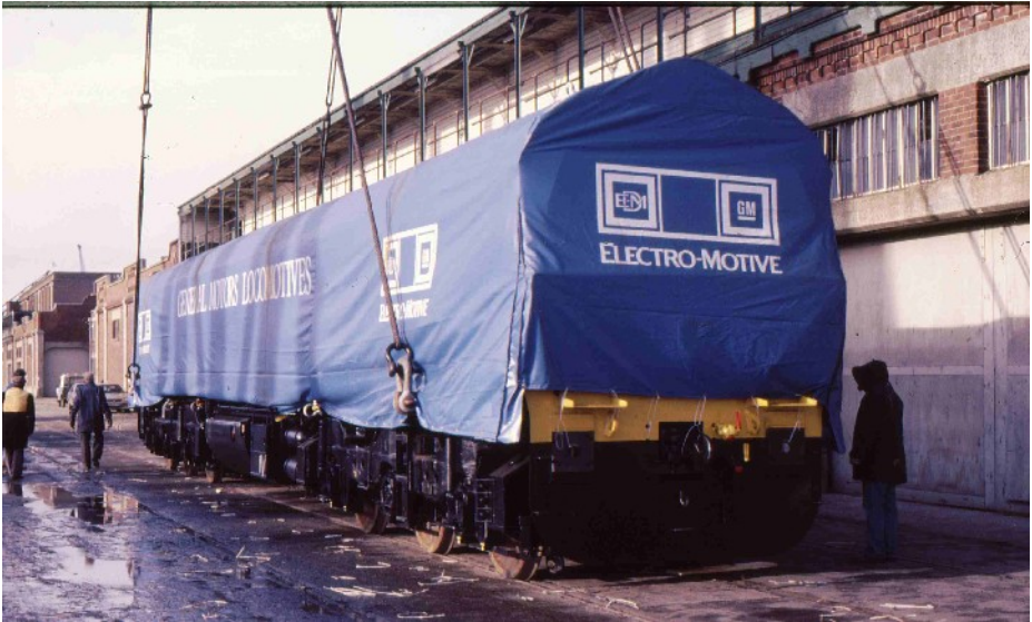
Having been lowered on to its bogies, 59002 is ready to be unhooked from the crane and be prepared for service.
