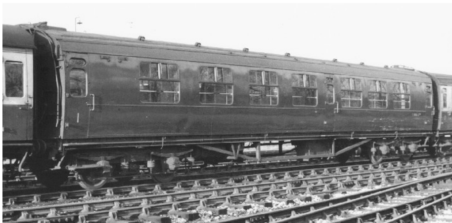
A typical later pattern Bulleid CK, thought to be one of the loose coaches ordered in August 1947 and constructed between 1948-51 Photo Mike Stollery collection
