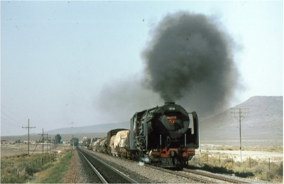
Former condensing North British 1954 built class 25 4-8-4 No 3480 "Susie" storms through the Little Karroo semi arid desert with a northbound freight in 1981. All except three condensers were converted to conventional form between 1974 and 1979. Colin Stone
