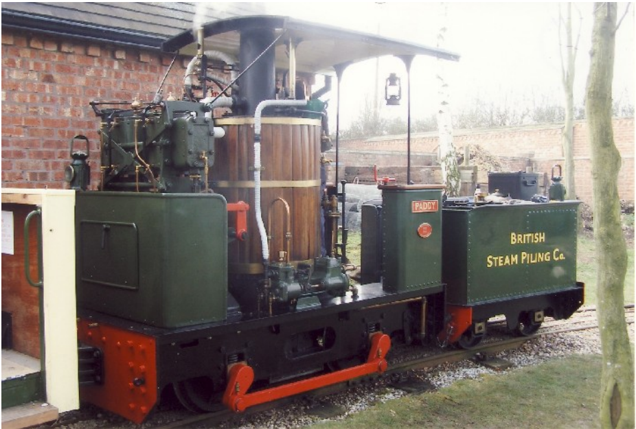
Paddy the replica De Winton vertical boyled locomotive.
