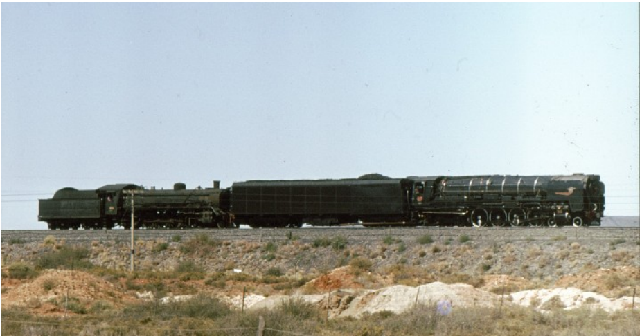
The last active SAR Class 25 Condenser (North British 1954) is seen in action in 1982 towing a condemned 19D 4-8-2 No 2536 (Borsig 1937) to De Aar locomotive dump. As can be seen in this shot No 3511's tender which contains some of the condensing gear is a few feet longer than the engine. Colin Stone
