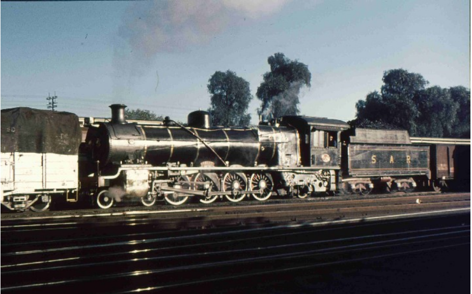
Also photographed in 1980 Beyer Peacock 1925 built class 15A 4-8-2 No 1970 named "Milly" shunts at De Aar. Her super shine condition is due to her being the depot "pet" and of being one of just three 15A's not reboilered to class 15AR Colin Stone
