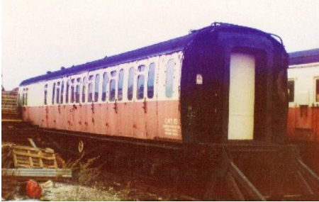
'Shorty' BTK 2850 showing its multi-door configuration in contrast to the more common BTK 4036 (right) carrying Chipmans No. CWT12, both photographed at Chipman's depot, Horsham September 1976. Behind 4036 is a Maunsell BCK, either 6697 or 6699, both now stored on the Swanage Railway. [photos Mike Stollery
