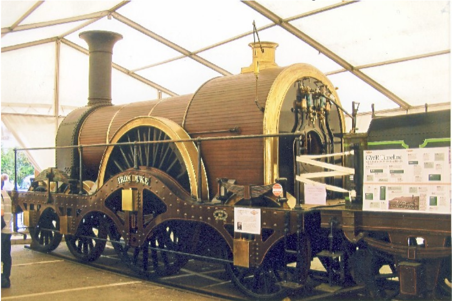
“Austerity” RSH 7135/1944, WD no.75185, seen here in her rebuilt form as the replica Broad Gauge IRON DUKE at the Gloucs-Warks Rly GWR 175 event held during May 2010. Photo: Steve Green.
