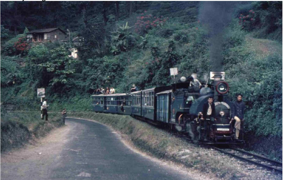
Darjeeling Himalayan Railway Class B 0-4-0T No 803 with the TEFS charter forming an extra fourth portion of the daily New Jaipalguri to Darjeeling train on 19 November 1975. Note:- The two chaps on the front of the loco are the hand sanders, the coal pusher/breaker is perched on the top of the loco behind the dome. Also note the TEFS members on top of the coaches and other TEFS lads "grabbing a phot" before leaping back on board the moving train. Colin Stone
