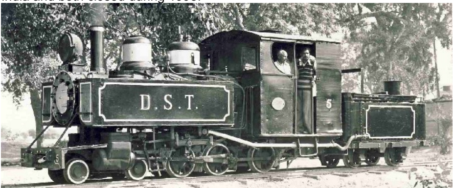
Daurala Light Railway No5 (Unidentified) was modified with a four wheeled tender. This location kept its locomotives in immaculate condition as seen in this 1978 view.
