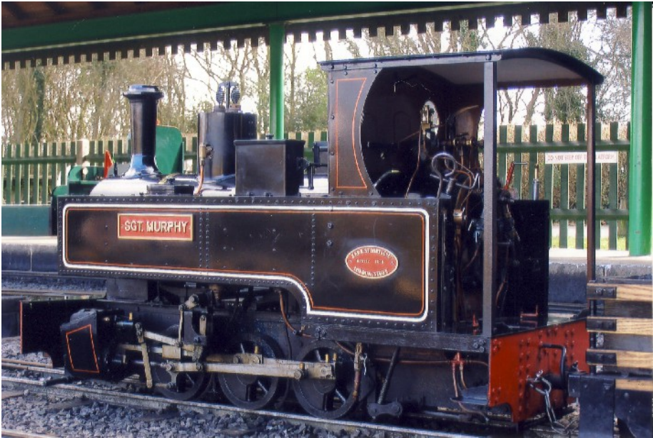
Preserved KS 'Haig' class 0-6-0T SGT. MURPHY, in original condition? No, not quite! It's actually a 7 ¼" gauge, 1/3 rd full-size scale model, based at the Eastleigh Lakeside Railway. Steve Green
