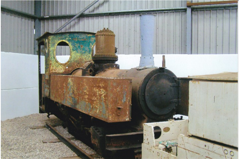
Henschel 14928 (Marromeu No.3) seen inside the Statfold Barn's Grain Store in June 2012. Note this loco features straight side tanks.
