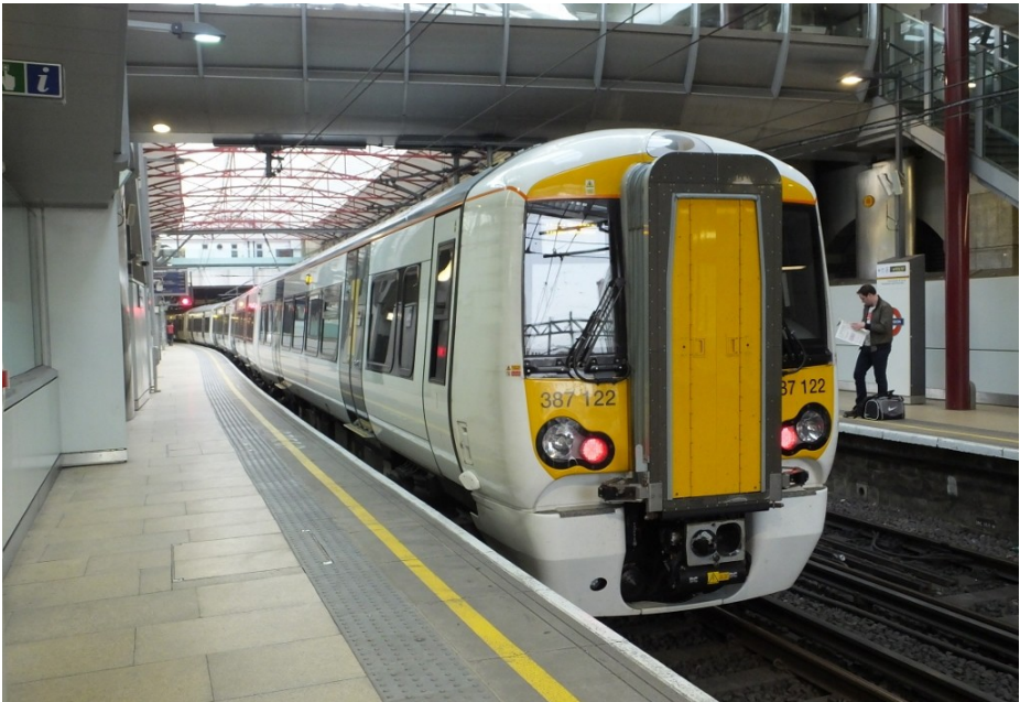
The newest trains on the network at time of writing are these class 387/1 units being delivered to Thameslink as an interim measure to release class 319 units to Northern Rail. They will in turn move on when the new Thameslink fleet is delivered. Ken Aveyard
