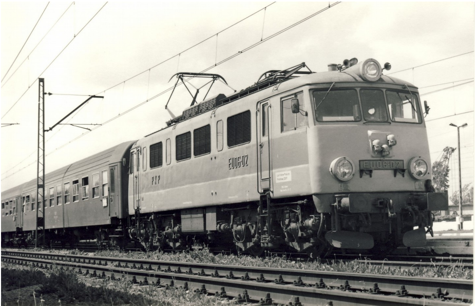
Polish Railways class EU06 locomotive EU06-02 built by English Electric as a derivative of the BR class 83 locomotive. Przeworsk 3rd June 1994 WRS archive
