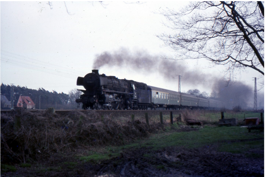
Class 012 Three Cylinder Pacific No 012-066 storms north past the village of Leschede with D714 express on April 18th 1975. Note how hard the loco' is being worked hard with the exhaust being thrown high out of the chimney. Colin Stone
