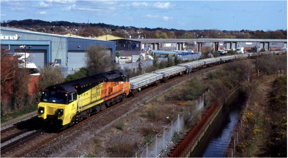
Colas Class 70 No 70809 heads a train load of new concrete sleepers to Upwey in conjunction with relaying the UP line in that area. See the article on Dorset mainline locomotive visitors 2015 on page 9. C Stone
