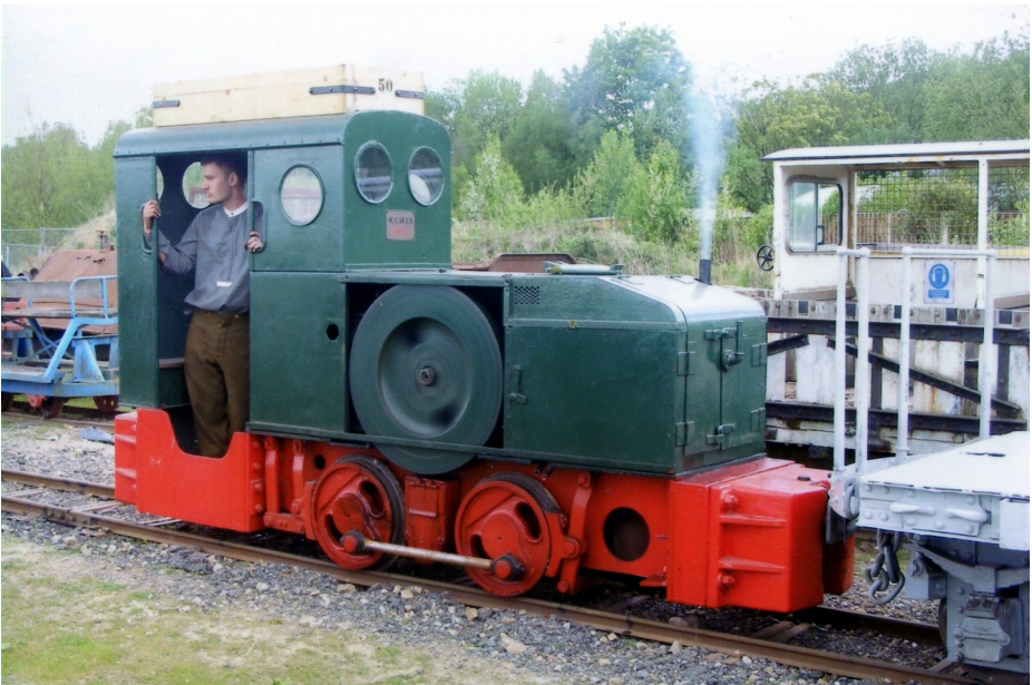
The Deutz loco. Note the very large fly-wheel, and "clag".
