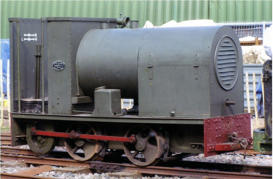
The strange McEwan-Pratt/Baguley 0-4-0PM. The driver has to stand up! See article on Tracks to the Trenches from page 10. Steve Green
