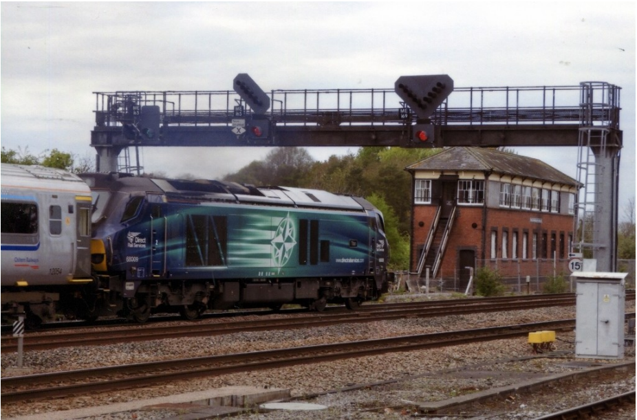
DRS 68009 “Titan” head a down service away from the station and pass the impressive, preserved signalbox. 68009 is one of a pair of class 68’s, the other being 68008, which are fitted with the necessary equipment to work the Chiltern and Scotrail passenger trains that run with DVT’s when their dedicated locomotives are unavailable.
