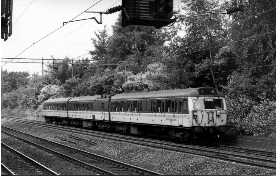
Regional Railways liveried Class 304 emu 304019 passes Heaton Chapel on 19 July 1994. Originally built as four car units for the Manchester to Crewe services most were reduced to three car by removal of the trailer composite. WRS P1641_5
