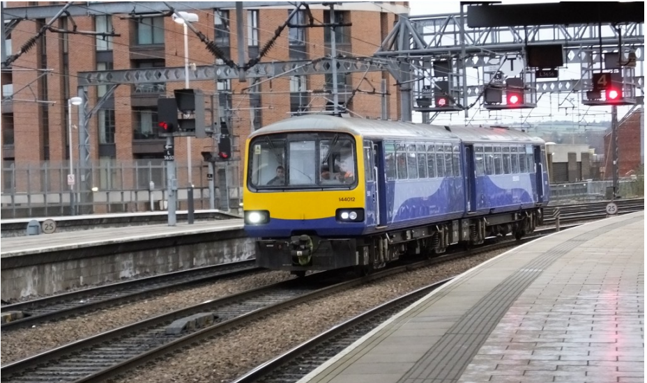
Class 144 Pacer unit 144012 is the unit modified by Porterbrook to meet the 2020 accessibility requirements. Destined to be a one off it is seen entering Leeds station on 3 January 2017. Robert Aveyard
