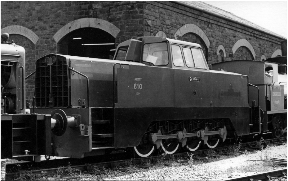
WD nos. 890 - 610 GENERAL LORD ROBERTSON is a 620hp 0-8-0DH Rolls Royce/Sentinel 10143/1963, AD class D2. Seen at the Avon Valley Railway 4 June 1989. WRS P1113_8
