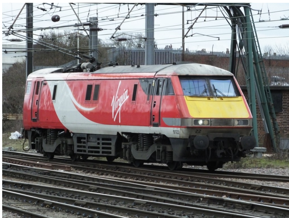
91122 running on three traction motors following snow damage is seen arriving at Doncaster West Yard light engine from Bounds Green en route to Wabtec where it will receive a replacement motor from fire damaged 91119. See article from page 6. Ken Aveyard
