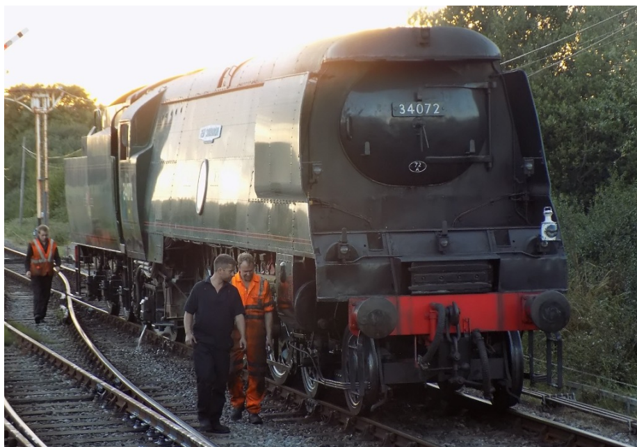
Battle of Britain No 34072 "257 Squadron" is seen at Harmans Cross being checked over for "hot boxes" during her test run . 09-08-2018 CS
