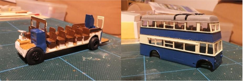
The Roe utility bodied Karrier trolleybus by Tiny Kits consists of a one piece body and a separate upper deck floor and seats as shown in the picture on page 20, with a combined chassis and lower deck.
