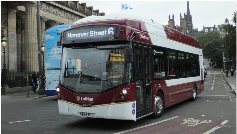
***In 2016 Wright introduced the Streetair a purpose designed all electric replacement for the electric versions of the Streetlight and Streetdeck. Only six were built, all single deck, entering service in Edinburgh in 2017 and these now see little use due to reliability and capacity issues. 284 is seen exiting The Mound and crossing in to Hanover Street.***
