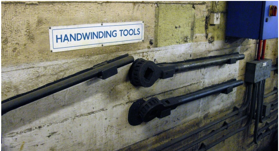
Heavy duty tools used to wind the escalators during maintenance.
