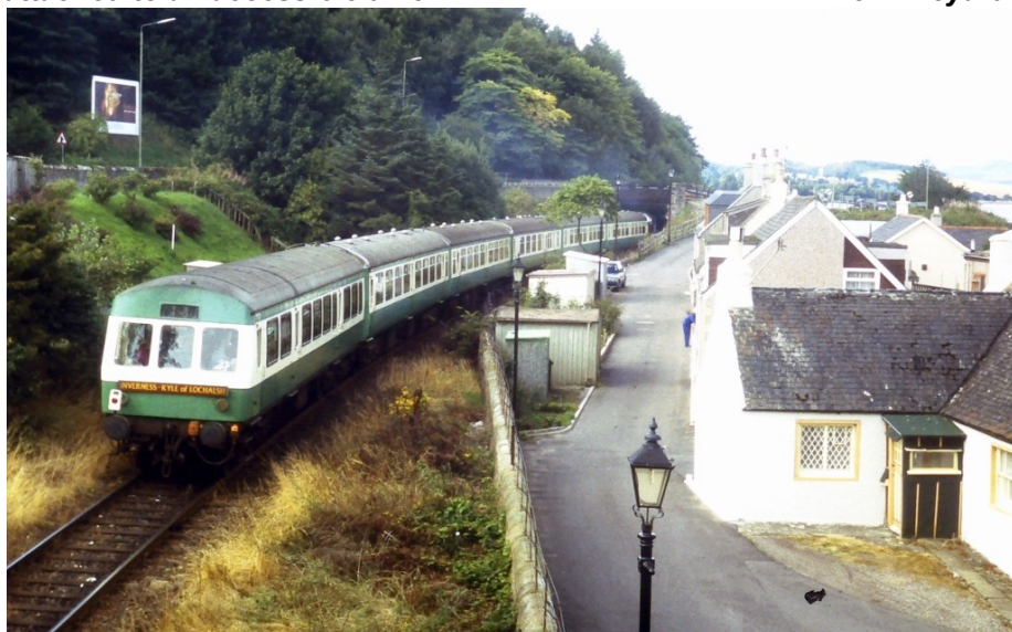
One final picture from Scotland. The observation coach mentioned on page 9, created from a class 101 driving trailer, is seen at Clacknaharry.
