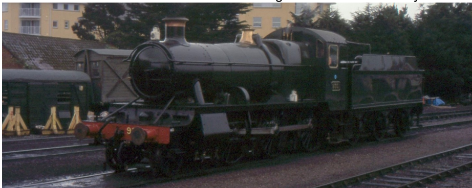
GWR 2-6-0 9351 a creation of a type the GWR never had being a tender version of the 51XX tank engines, using 5193 as the donor. K Aveyard
