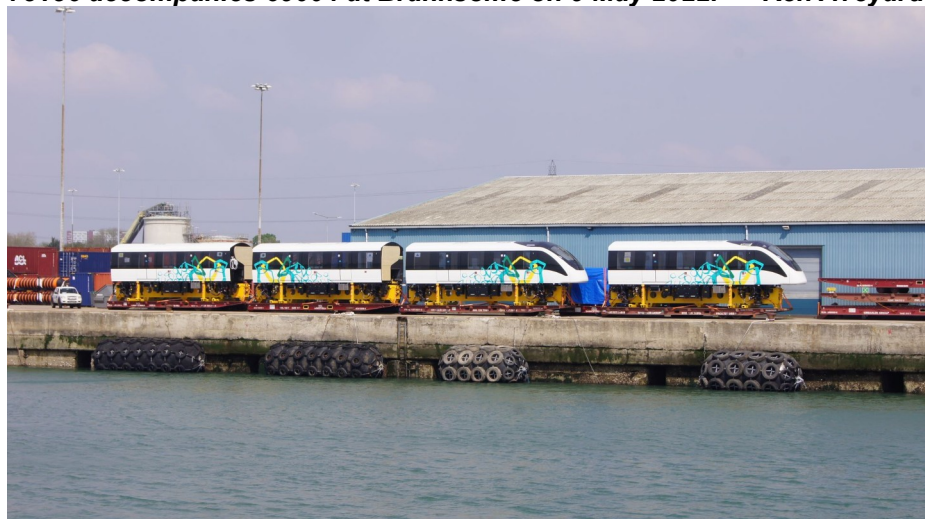
On 23 April 2022 Trevor Hargreaves took a boat tour around Southampton Docks and found these tram like vehicles on the dock side by the car loading berths. Notice they're held up by longitudinal girders under the centre of the bodies because these are new Monorail cars for Cairo, Egypt. They have been constructed at the Bombardier plant at Derby as part of an order for 70 four car sets, one of which is pictured above.
