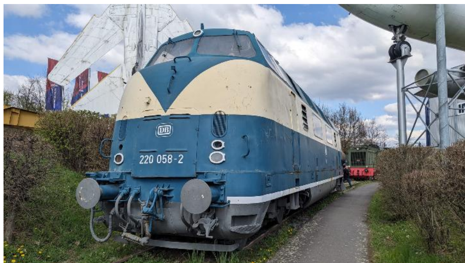
Diesel Hydraulics 220 - 071-5 and 220-058-2 at Speyer Museum in Germany. Originally V200 class built at MaK Kiel in 1956 and also at Krauss Maffei. Twin Maybach engines.
