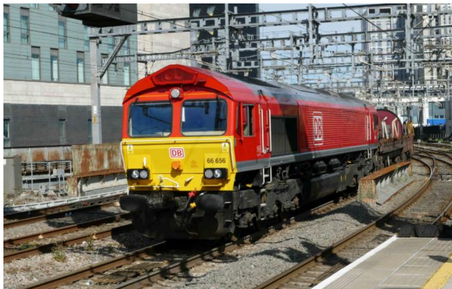
DB has re-gearred 10 class 66's for heavy haul services and these have become quite common on steel trains through Cardiff. Here 66656 heads west on 16 April 2025.
