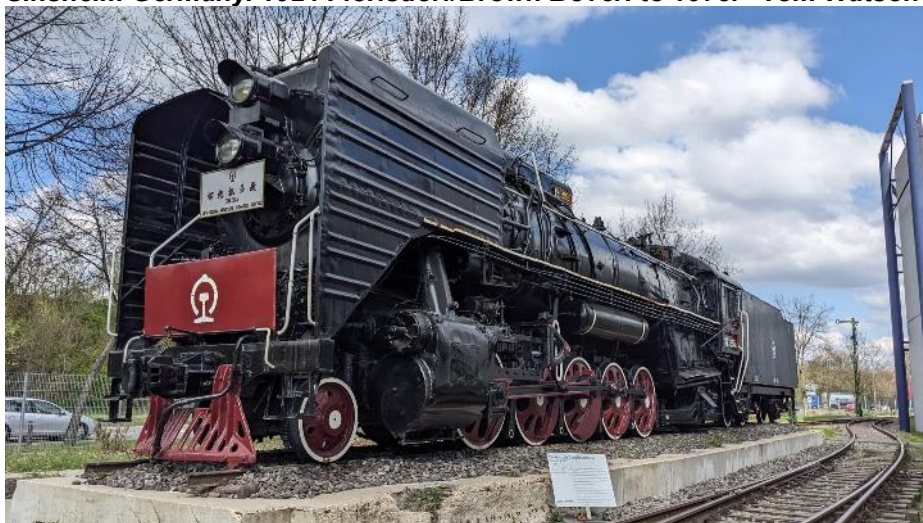
Chinese QJ 2-10-2 at Sinsheim. Only Chinese loco in Germany. One of over 5000 built at Datong. Originally preserved in Lucerne but too big to travel by rail or road so it was transported by road - on its side!!
