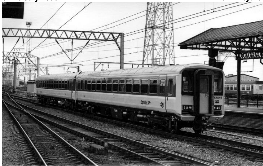
The class 153 units were formed from the splitting of the 155 2-car sets. Here 155333 which became 153333 and 153383 is seen arriving at Crewe from Cardiff on 2 July 1988. WRS P1011_6
