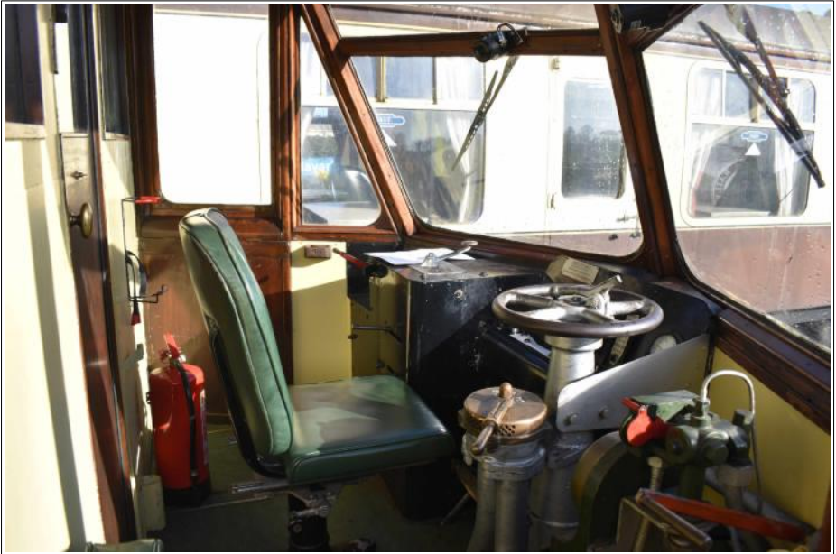
A view of the drivers cab. Note the central driving position.
